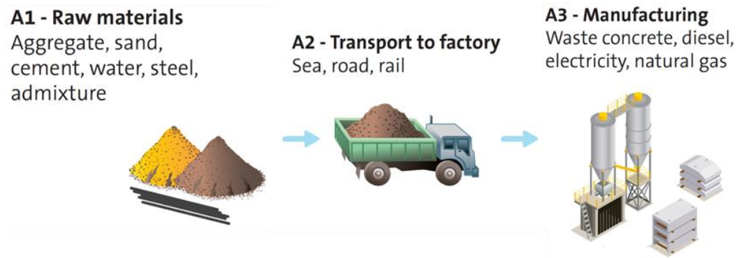
Figure 1 – Cradle-to-gate (A-A3) life cycle stages of precast concrete products
